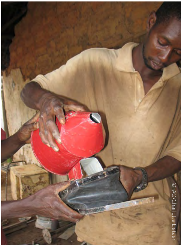
Image 7: A welder in Sierra Leone making a locally-made smoker (left) and the completed smoker (right)
